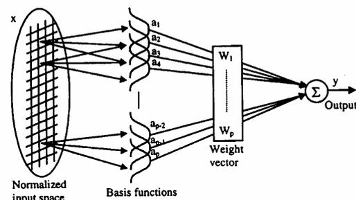
Figure 2. Typical structure of a neurofuzzy network (Brown and Harris 1994).
