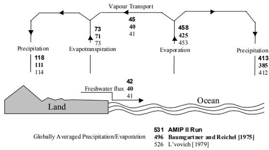
**Figure 2.** Comparison of annual mean components of global hydrological cycle with observation-based estimates. The units are 10<sup>3</sup> km<sup>3</sup>/year.
