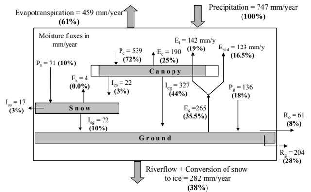
**Figure 4.** Mean annual values of inputs, outputs, and moisture exchanges to, from, and between the three moisture reservoirs over land in mm/year and as a percentage of annual precipitation.
