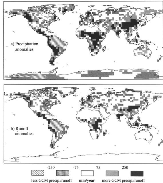
**Figure 3.** Differences between model and observed, mean annual precipitation and runoff estimates over land (mm/year).
