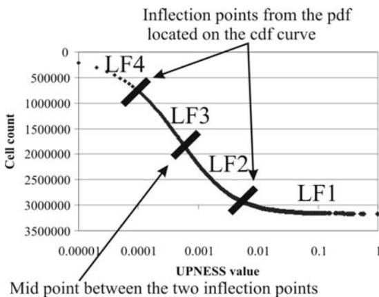
**Figure 2.** The UPNESS index cdf plotted on log scale showing three points discriminating the four-landform elements.
