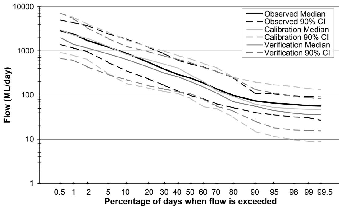
**Figure 3.** Observed (1/1/1950 – 31/12/1998) and modelled runoff for the calibration (1/1/1950 – 31/12/1969) and verification (1/1/1970 – 31/12/1998) period's median annual flow duration curves, with 90% confidence intervals.
