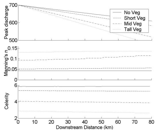
**Figure 8.** Downstream peak discharge attenuation (50yr ARI inflow) with roughness (middle axes) and wave celerity
