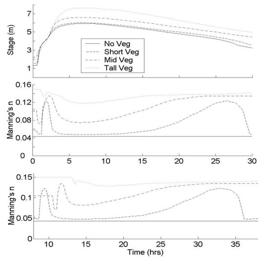
**Figure 7.** Sample variation of input stage vs time for the 50yr ARI inflow hydrograph (top); corresponding variation of Manning's n at 0km (middle) and 50km (lower) for each veg.
