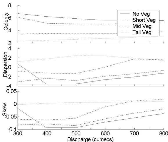
**Figure 6.** Wave celerity, dispersion coefficient and average changes in skew for hydrographs with peak discharges from 300 to 800 cumecs.
