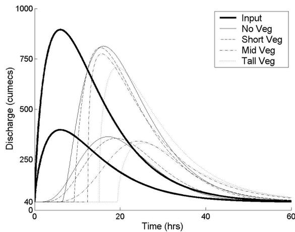
**Figure 5.** Selected input hydrographs (2yr and 100yr ARI) and the corresponding fitted hydrographs at 60km downstream for each vegetation scenario.
