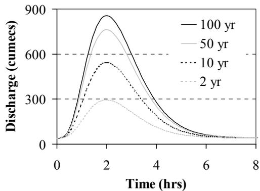
**Figure 2.** Input hydrographs designated by return interval.
