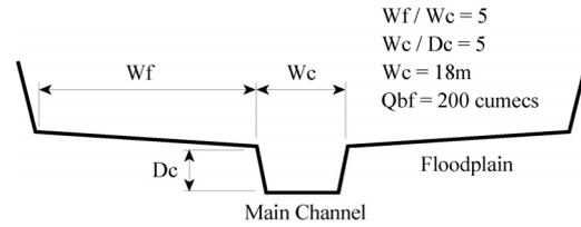
Figure 1. Cross-section schematic with dimensions.
