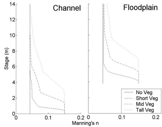
**Figure 4.** Main channel and floodplain roughness profiles for each test scenario.
