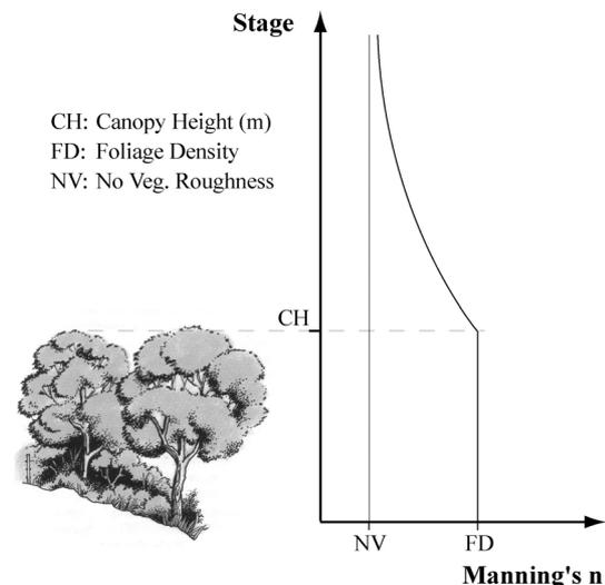
**Figure 3.** Shape function for the variation of vegetal roughness with flow stage.
