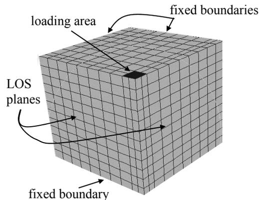
**Figure 2.** Footing mesh using ABAQUS.
