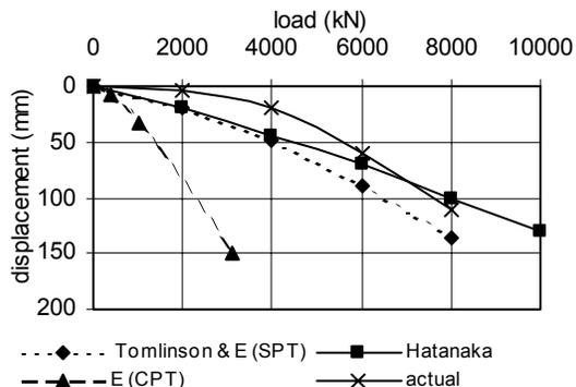
**Figure 7.** Load-deflection curve for 3 m south footing.
