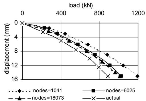
**Figure 5.** Load-deflection curve for N=50.
