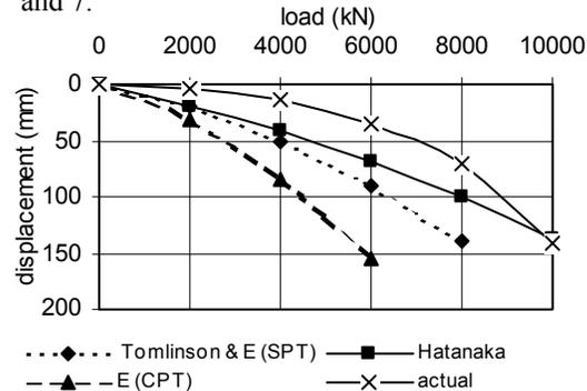
**Figure 6.** Load-deflection curve for 3 m north footing.
