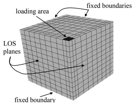
**Figure 2.** Footing mesh using ABAQUS.
