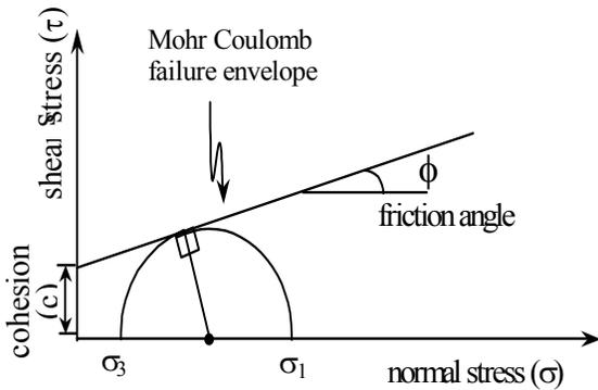
**Figure 3.** Mohr Coulomb's failure surface.
