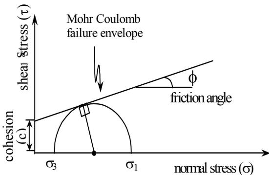
**Figure 3.** Mohr Coulomb's failure surface.
