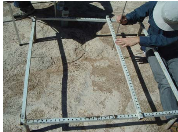
Figure 3. The instrument for measuring the microDEMs in use.
