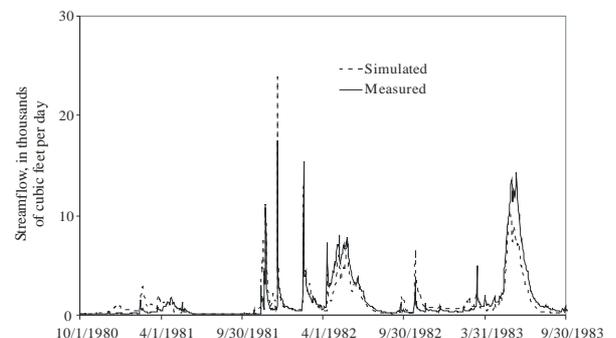
**Figure 2.** Comparison of simulated and measured streamflow at the outlet of Sagehen basin
