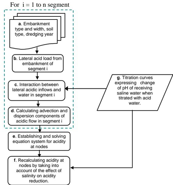
**Figure 3:** Flowchart of calculation in acidity module
