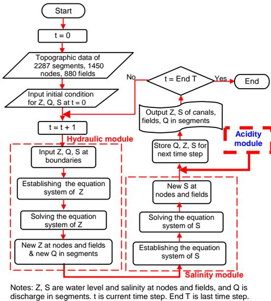
**Figure 2:** Incorporation of acidity module into VRSAP model
