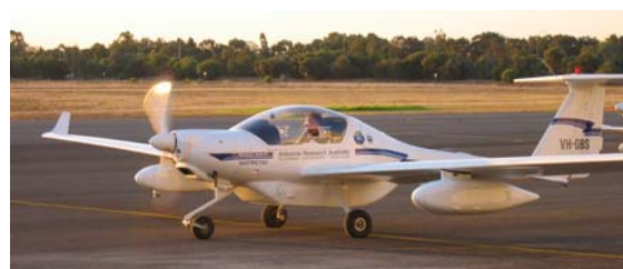
Figure 5. The Diamond ECO-Dimona aircraft with PLMR mounted under the fuselage, and thermal imager, digital camera and NDVI scanner in an underwing pod.
