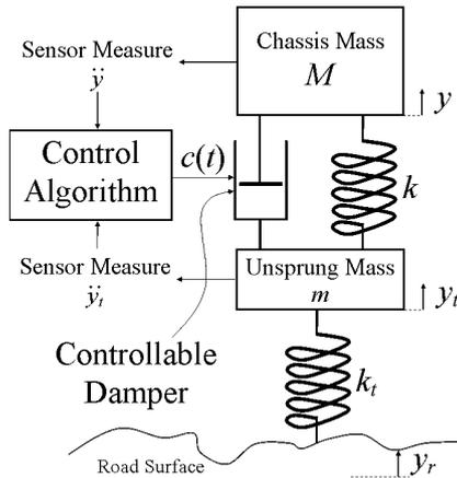
**Figure 1.** Semi-Active Suspension
