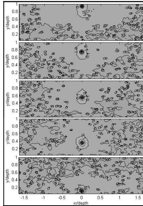
**Figure 6.** Y-velocity correlation plots at 5 depths in the flow ( $y = 0.11h, 0.36h, 0.55h, 0.75h$  and  $0.94h$ ) for the first of the 11 fields.
