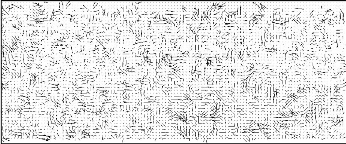
**Figure 4.** Part of a velocity field obtained from a PIV analysis. Note that the mean velocities (for each horizontal line of data points) have been removed from the plot to show the flow structures. Note that the top 10 lines are above the water surface and appear in the data due to reflections from the water surface.
