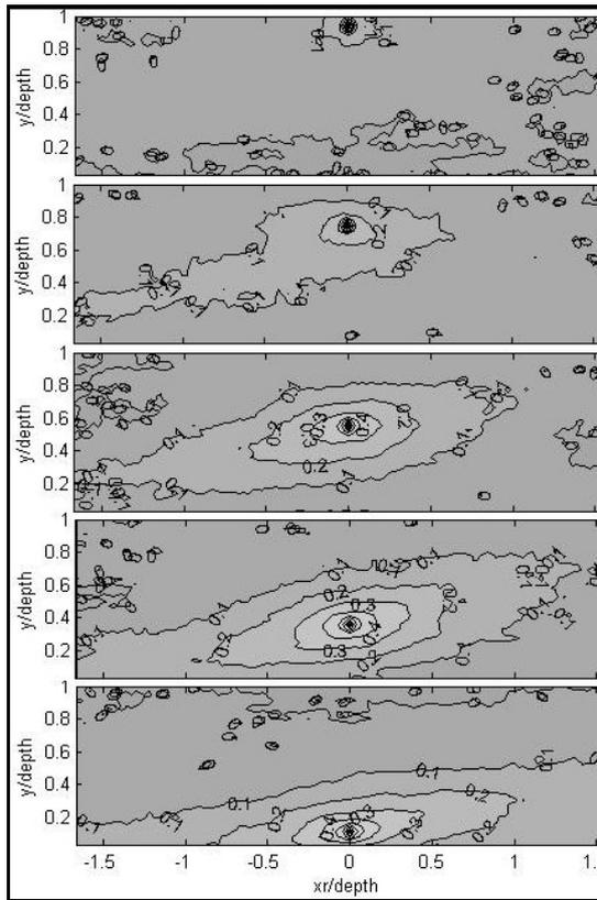
**Figure 5.** X-velocity correlation plots at 5 depths in the flow ( $y = 0.11h, 0.36h, 0.55h, 0.75h$  and  $0.94h$ ) for the first of the 11 fields.
