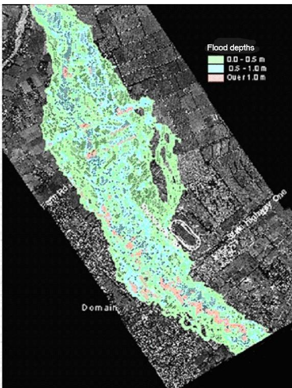
**Figure 2.** Map showing extent of flood inundation for the estimated 200 year return period event for Ashburton, New Zealand (Modelled using Hydro2de with a 10 m grid of 370,000 points).
