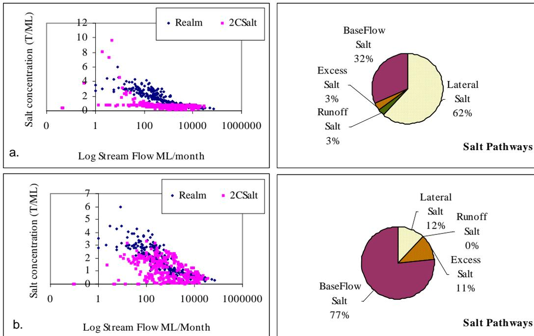
**Figure 5. Comparison of flow-concentration and salt pathways for a) current b) developmental salt pathways of 2CSalt model**
