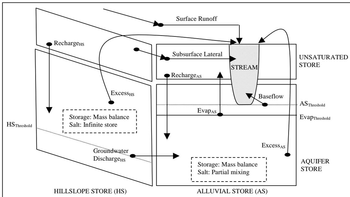
**Figure 1. Pathways of water and salt movement in the 2CSalt model**
