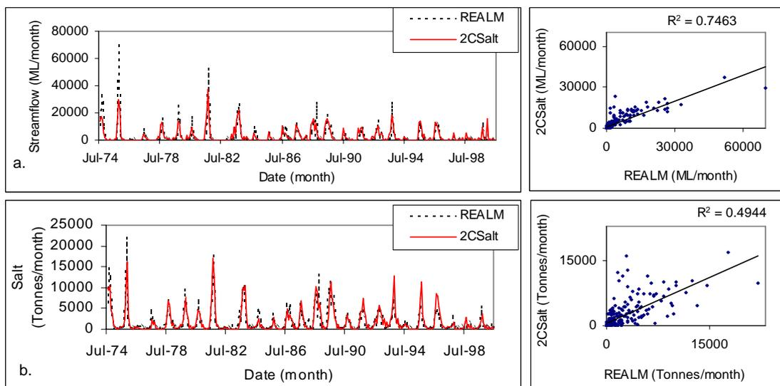
**Figure 3. Comparison of REALM and 2CSalt end-of-catchment a) stream flow (ML/month) and b) salt export (tonnes/month).**
