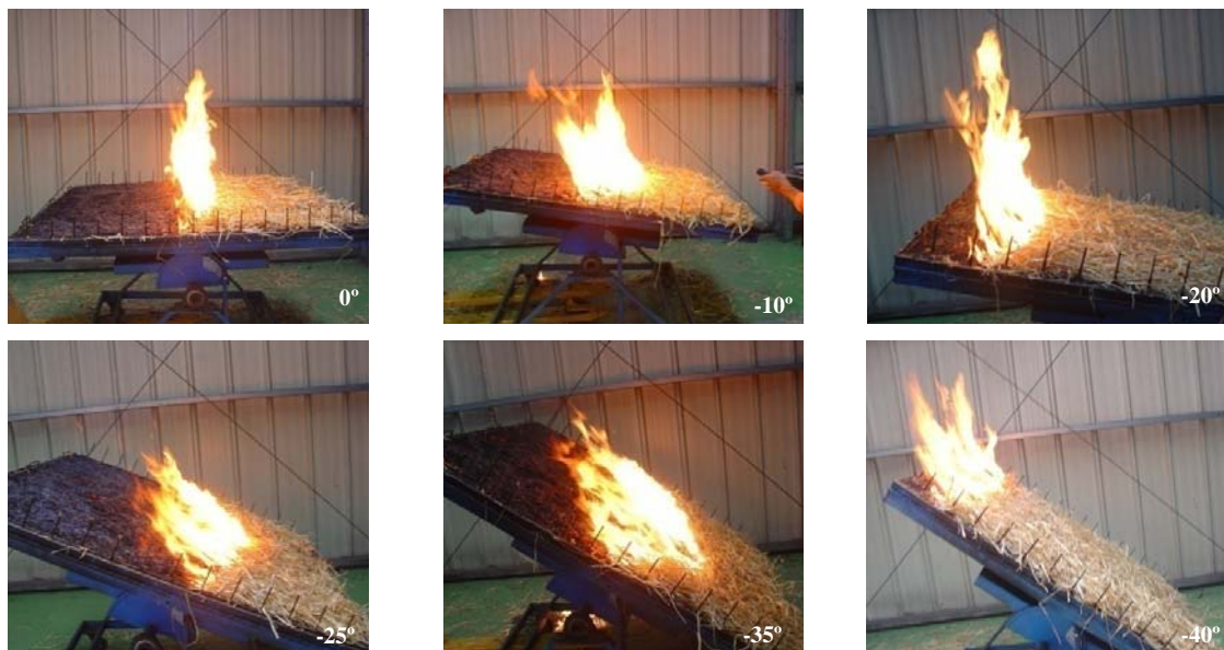
Figure 4 – Flame geometry for tests with variable slope from 0^\circ \leq \alpha \leq 40^\circ . The variation of the flame length and flame angle for different slope angles can be observed (Fuel: straw; Fuel load: 0.6 \text{ kg/m}^2 ).
