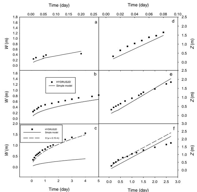
**Figure 2.** Penetration of wetting front horizontally into the bed from the edge of the furrow ( $W$ ); a) sand, b) loam (lower time scale used), and c) clay, and the vertical penetration below the furrow ( $Z$ ); d) sand, e) loam and f) clay. The second line for the clay is where a different value of  $S$  was used (see text). Note different time and length scales are used.
