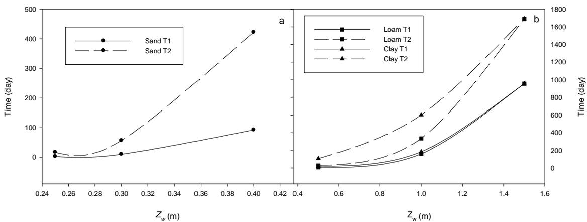
**Figure 4.** Depth of the watertable ( $Z_w$ ) with time for solutes to reach the soil surface (T1) and increase to  $100 \text{ mmol m}^{-3}$  (T2); a) sand soil and b) loam and clay soil. Note different scales on both axis in each panel.
