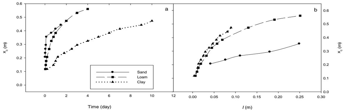
**Figure 3.** Washout distance ( $X_c$ ) with a) time and b) cumulative infiltration ( $I$ ) for sand, loam and clay soils.
