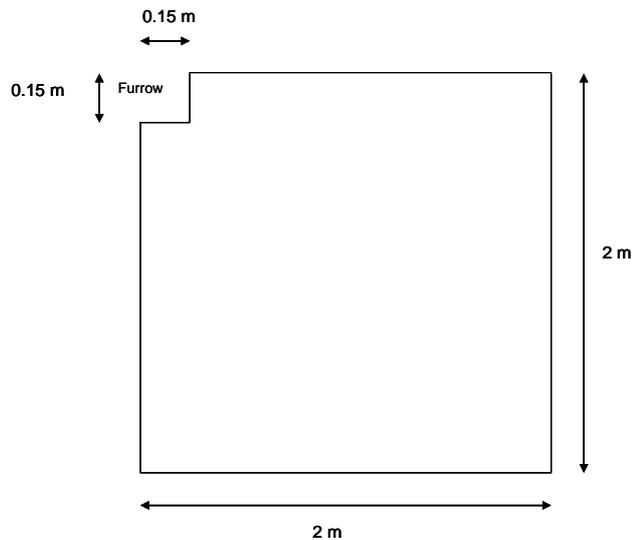
**Figure 1.** The domain used in the generic modelling simulations. No flow boundary conditions occur on the right hand vertical boundary and on the left hand vertical boundary below the depth of the furrow.
