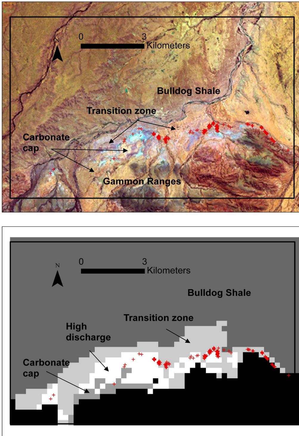
**Figure 2.** Public House Springs study area using Landsat false colour image (upper panel) with Bands 7 (red), 3 (green) and 1 (blue) to illustrate differences between evaporative discharge units. The lower panel shows the distribution of five classes of evaporative discharge using a 250x250 m cell size. The position of spring vents are shown as small red crosses and areas of blue-white in the upper panel are due to salt deposition in the high discharge zone.
