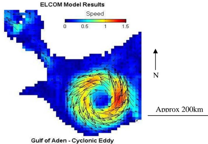
**Figure 6.** Cyclonic eddy prediction. Left hand figure is sourced from Bower & Fratantoni, 2002. Units on right hand figure are metres per second
