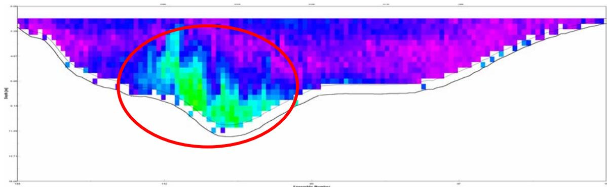
**Figure 7.** ADCP field data at lagoon exit. The bottom contour offset is the approximate zone of bed penetration of the ADCP beams.
