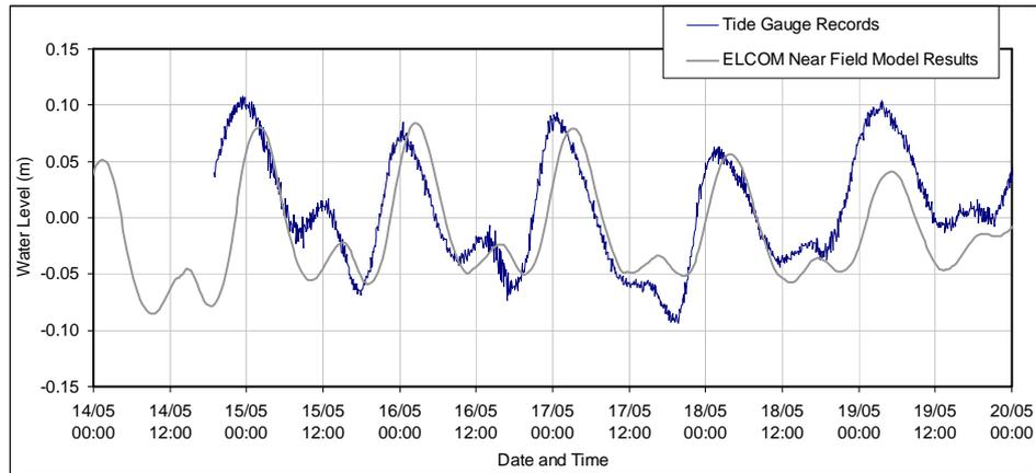
**Figure 4.** Nested model tidal calibration example.
