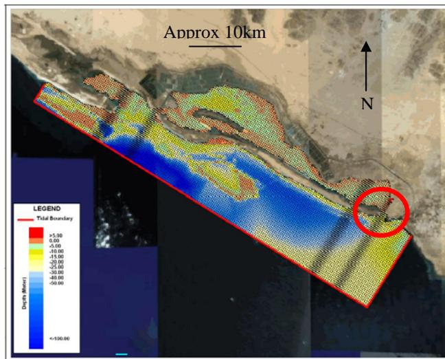
**Figure 2.** Nested model bathymetry. Red circle shows density current location (section 4). Photo from Google Earth
