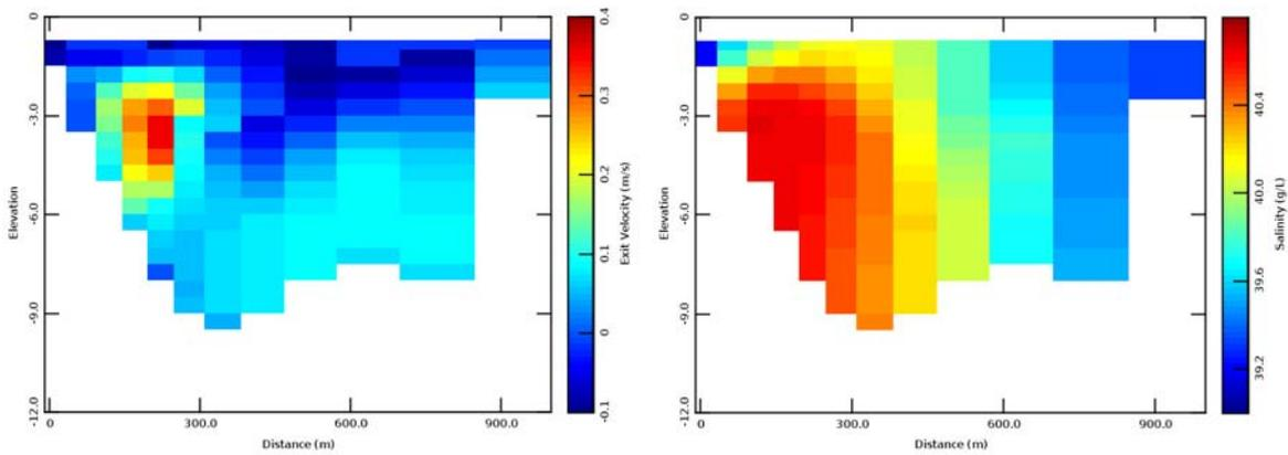
**Figure 8.** Density current exiting the fringing lagoon: model bottom layer data.
