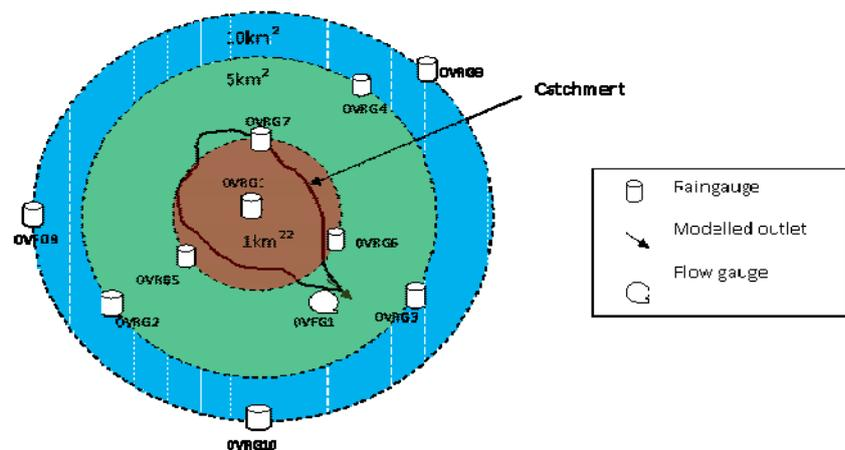
Figure 1. Schematic of the layout of the catchment and rain/flow gauges
