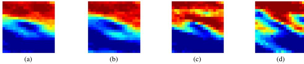
Figure 3. Layer 4 after model inversion with diffraction tomography by SNOPT (a) and GPS (b), and with traveltome tomography by HJDS (c) and GA (d). The genetic algorithm, because of its global nature, does not require initial guess.
