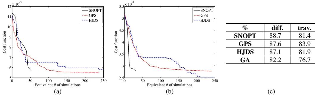
Figure 4. Performance results for the local optimizers (SNOPT, GPS and HJDS) in the model inversion with diffraction and traveltome tomography, (a) and (b), respectively. In both cases one complete observable simulation takes 43 seconds; thus, 250 equivalent simulations require approximately 3 hours of computing time. In the table in (c) we present the percentage of cells where the model is inverted correctly, both with diffraction (diff.) and traveltome (trav.) tomography.
