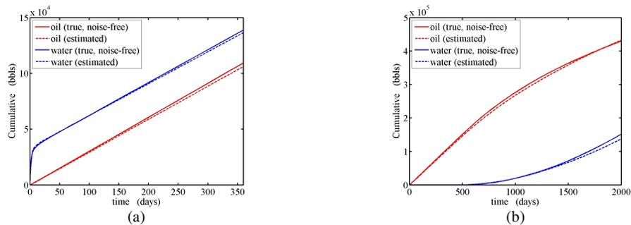
Figure 5. (a) Oil production and water injection forecast (360 days) for the solution obtained by SNOPT and diffraction tomography. (b) Oil and water production forecast (2000 days) for the recalibrated (first 1000 days) solution. In both cases the results are compared with those obtained for the true model  $\mathbf{m}^*$ .
