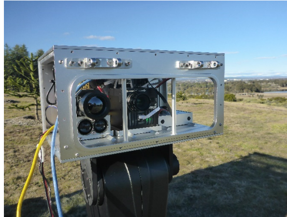
Figure 4. The ANU forest spectroscope in the first operational field trials in August 2017. Note that external casing is removed here and that the SWIR camera was not installed.
