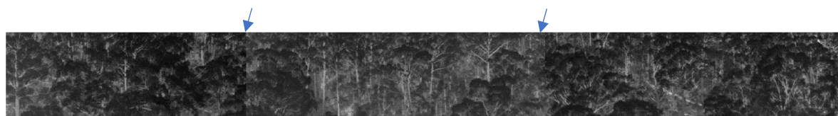
Figure 3. A panorama thermal image of the forest canopy. This image shows two of the LWIR sensor artefacts that have caused some difficulty in data analysis as noted in the text. The step changes in the image brightness (at arrows) are caused by the automatic image adjustment made by the camera.
