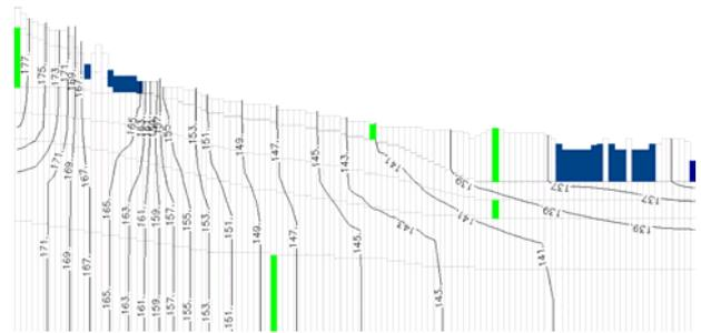
Figure 6: Steady state model simulation results: distribution of hydraulic head (mASL) (observation points marked in green).
