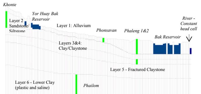
Figure 5: Spatial discretisation of model domain and location of head observation points (green cells), reservoirs and the River (blue cells).
