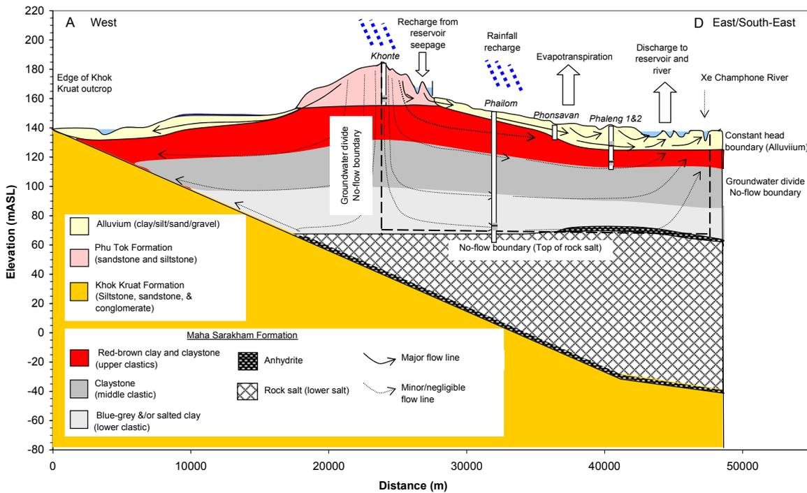
Figure 3: Conceptual groundwater flow model
