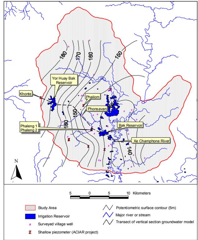
Figure 4: Potentiometric surface for shallow aquifer and location of model transect and all monitoring points.
