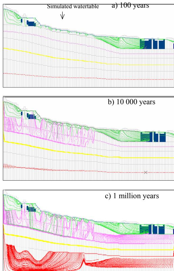
Figure 7: Forward and backward particle tracking for steady state simulation over a) 100, b) 10 000 and c) 1 million year periods. Coloured lines correspond to simulated flow paths of particles placed in Layer 1 (green), Layer 4 (pink), Layer 5 (yellow) and Layer 6 (red).
