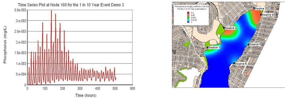
Figure 4. Example of output: time series plot at a node and contour plot of concentrations.
