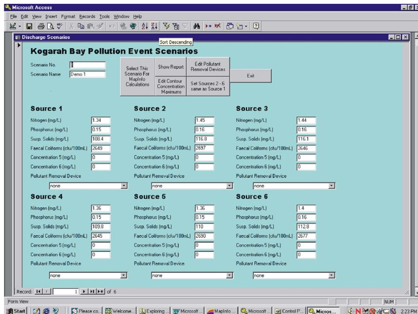
Figure 3. Database input screen used to create scenarios and edit parameters
