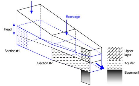
**Figure 1:** Representative diagram of the Flowtube model. Source: (Argent, 2001)
