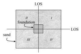
Figure 1: Lines of symmetry for square footing.
