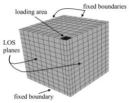
Figure 2. Footing mesh using ABAQUS.
