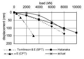
**Figure 7.** Load-deflection curve for 3 m south footing.
