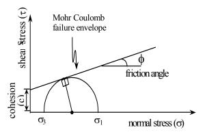
Figure 3. Mohr Coulomb's failure surface.
