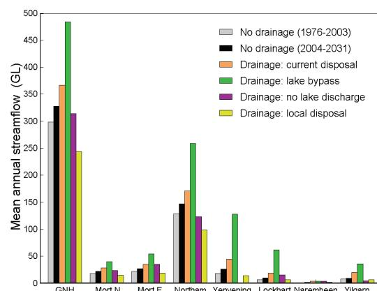
**Figure 1.** Predicted mean annual streamflow (2004–2031) at eight key locations in the Avon catchment for a variety of drainage scenarios.
