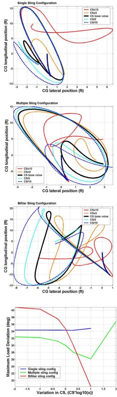
**Figure 6** Plan view of load oscillation, and maximum load deviation for variation in load side force coefficient (CS)
