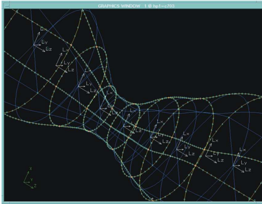
Figure 2. Meshable geometric representation of the flow domain (empty mesh) around an eccentric stenosis (magnified)
