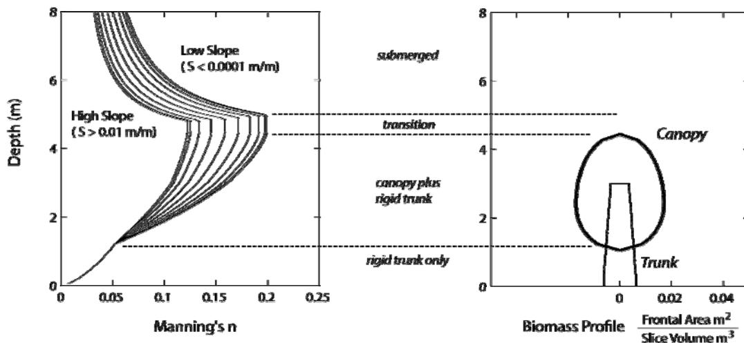
**Figure 1** Sample ROVER roughness profiles for a tree constructed from trunk and canopy characteristics.
