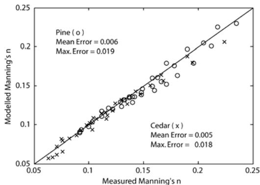
**Figure 8** Comparison of modelled and measured roughness values.
