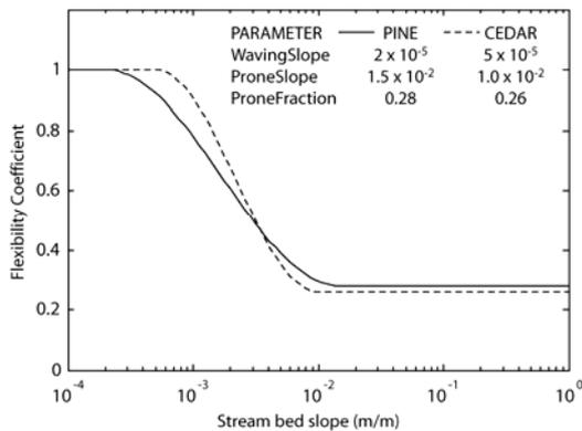
**Figure 7** Optimised ROVER flexibility function plots and parameters for pine and cedar.
