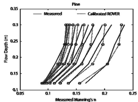
**Figure 5** Measured and modelled flow resistance (Manning’s *n*) versus flow depth isovels. Flow velocity of left-most curve is 0.9m/s, decreasing in 0.1m/s increments down to 0.1m/s at right.
