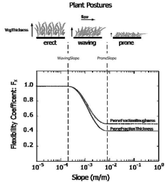
**Figure 3.** Schematic showing the relationship between the slope-based flexibility model (graph) and the behaviour of a grass sward (top).
