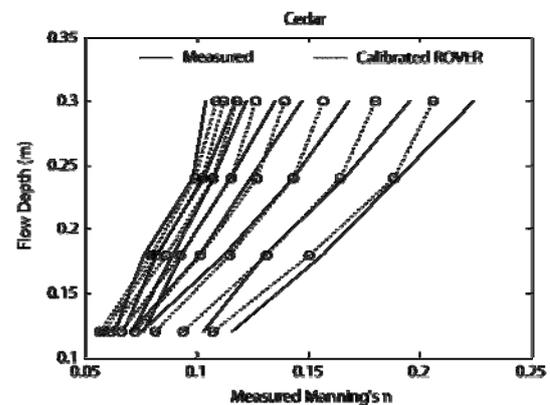
**Figure 6** Measured and modelled flow resistance (Manning’s *n*) versus flow depth isovels. Flow velocity of left-most curve is 0.9m/s, decreasing in 0.1m/s increments down to 0.1m/s at right.
