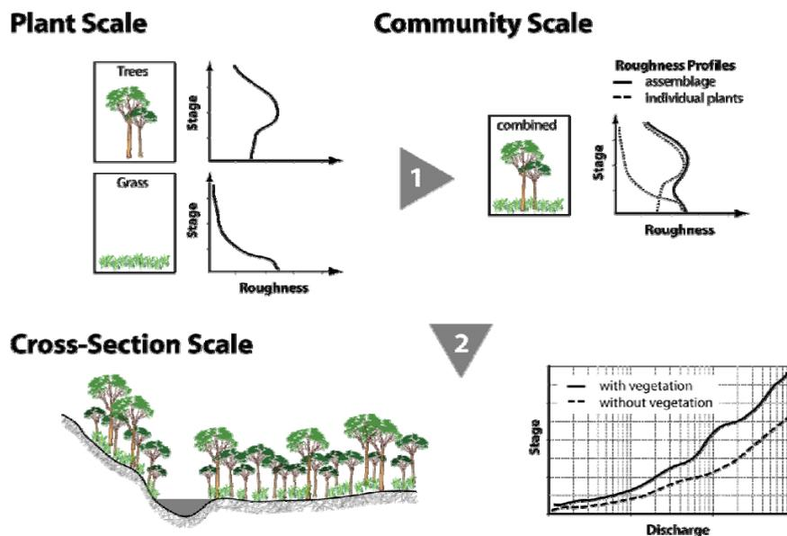
**Figure 2.** Structure of the ROVER model: plant-scale roughness profiles are defined then combined to provide a community profile. The distribution of plant communities around the cross-section then allows for estimation of the stage-discharge relationship.
