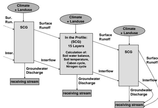
**Figure 3.** Model routing scheme of WASMOD with lateral transport (Kralisch et al. 2003).
