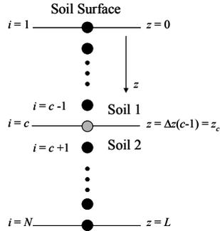
**Figure 1.** Grid system for 1D layered soil profile.
