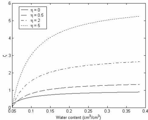
**Figure 3.** Relative gradient ratio ( $\zeta$ ) vs water content ( $\theta$ ) over the full wetting range for  $\eta = 0, 0.5, 2$  and  $5$ .
