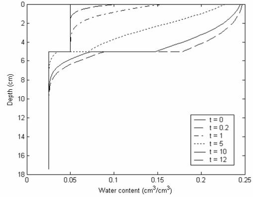
**Figure 2.** Water content ( $\theta$ ) profiles over depth for the non-linear transformation given by (16) with  $\lambda = \mu = 0.5$ .
