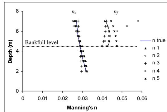
**Figure 5.** The true roughness and computed roughness versus depth when data contained noise (5 noisy data samples)
