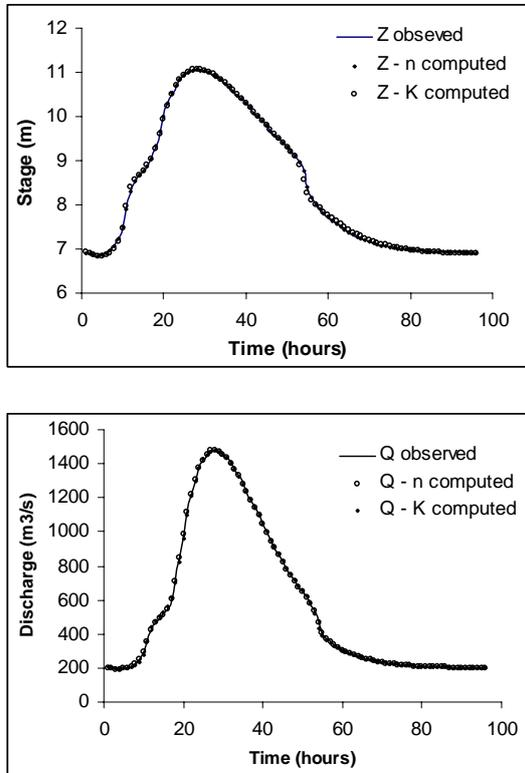
**Figure 7.** Observed hydrographs computed from the true roughness function and simulated hydrographs computed from the computed roughness functions and computed conveyance function
