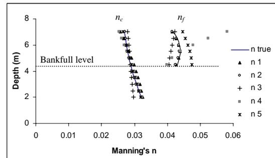
**Figure 1.** The true roughness and computed roughness versus depth when data contained noise (5 noisy data samples)
