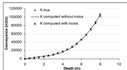
**Figure 2.** The true conveyance and computed conveyances versus depth when data with and without noise
