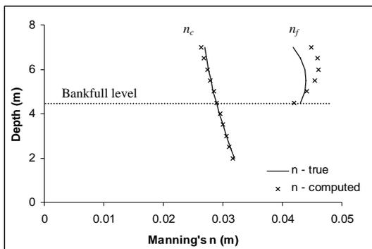
**Figure 4.** The true roughness and computed roughness versus depth when data contain no noise
