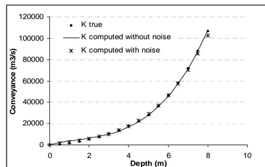
**Figure 6.** The true conveyance and computed conveyances versus depth when data with and without noise
