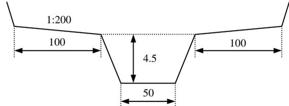
**Figure 3.** The cross section of the compound channel
