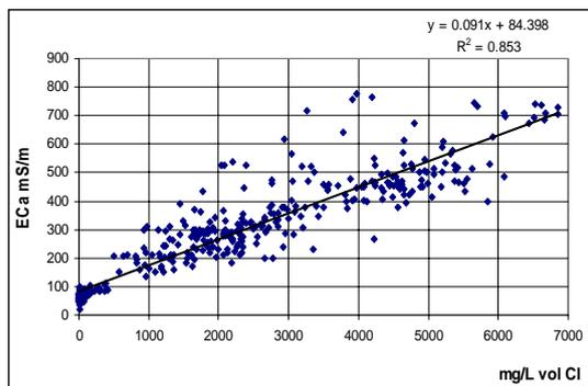
**Figure 3a.** Positive correlation between apparent electrical conductivity and salt (chloride) load.
