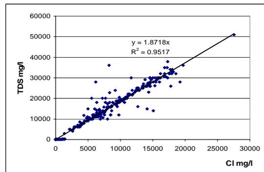
**Figure 3b.** Positive correlation between total dissolved solutes and chloride concentrations in the pore fluids.
