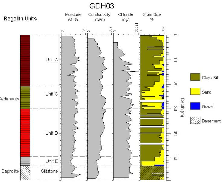
**Figure 2.** Visual display of drill log information of core hole GDH03 showing the stratigraphic units, geophysical logs and regolith attributes.
