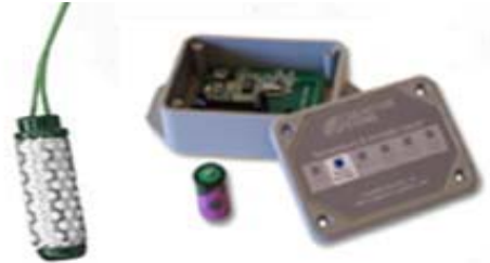
Figure 2: Soil moisture sensor and WSN unit with microprocessor, transmitter, battery and built-in sensors for monitoring atmospheric temperature and humidity.
