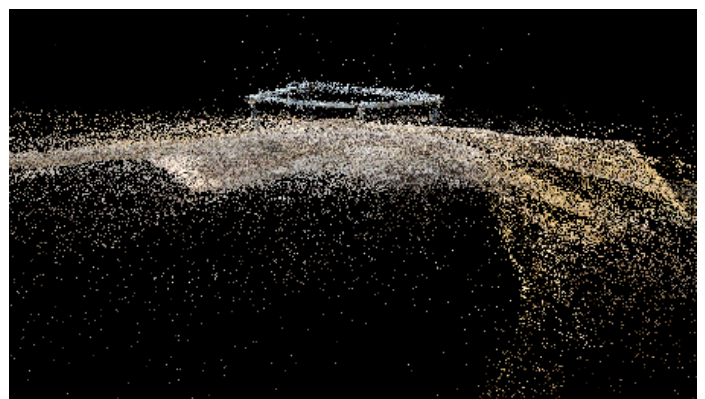
Figure 6. Photosynth point cloud (from northwest) illustrating the 3D depiction of the quadrat frame that was used to obtain the control points for the transformation.
