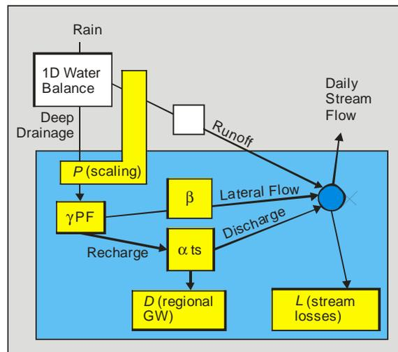
**Figure 1:** Simplified flowchart of conceptual model (calibration parameters shown in yellow).
