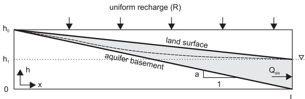
**Figure 2:** Idealised groundwater analogue of sloping aquifer, with surface head drop ( $h_0-h_1$ ) over the flow length ( $L$ ), and aquifer thickness at the outlet ( $h_1$ ). [from Walker *et al.* (in prep)].
