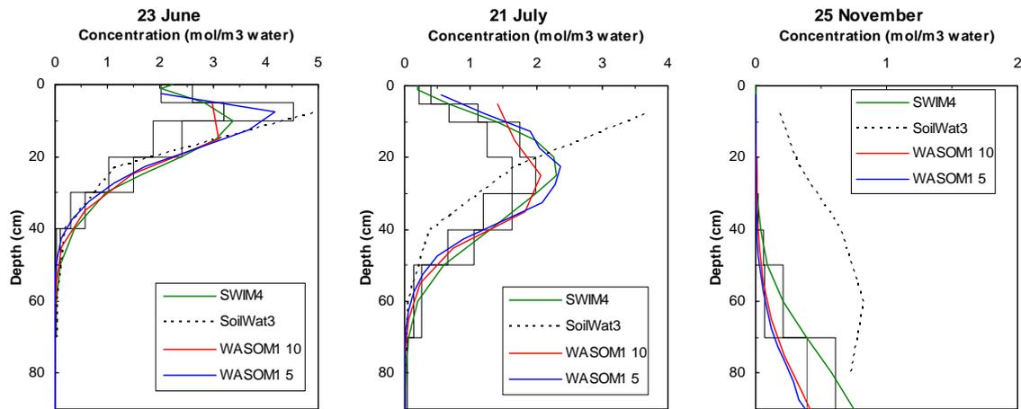
**Figure 4:** Comparison between WASOM1 and experimental (shown as histograms of 95% intervals around the mean for each depth interval) and modelling results from Verburg (Verburg 1996).
