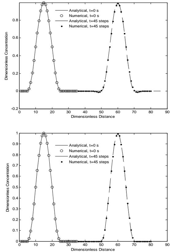
**Figure 2.** Numerical and analytical solutions for the translation of a sine-squared wave using QUICKEST (top) and ULTIMATE QUICKEST (bottom).
