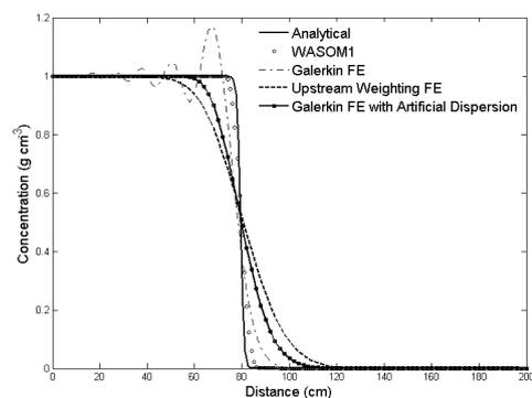
**Figure 1.** Analytical and numerical solutions for the transport of a tracer. Finite Element (FE) solutions obtained from HYDRUS (Simunek *et al.* 2005).
