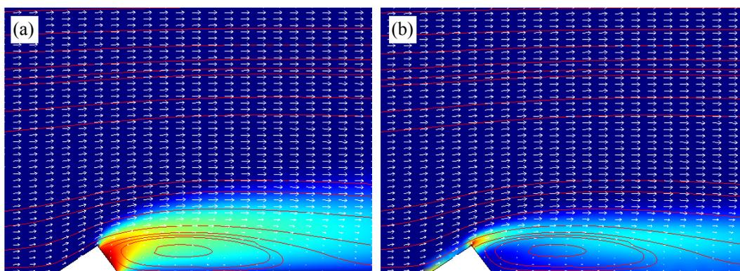
**Figure 7.** Results from the two-dimensional simulations: (a) logarithmically-transformed temperature field, (b) turbulent kinetic energy. White arrows indicate wind vector and red contours are streamlines.
