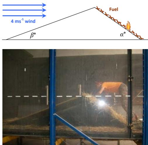
**Figure 3.** Schematic diagram (cross section) of the experimental ridge configuration and the approximate ignition point (top), and actual combustion tunnel set-up (bottom).
