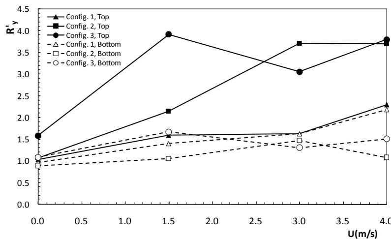
**Figure 5.** Nondimensional average values of the rate of lateral spread of the fire front at the top and at the bottom of the hill as a function of wind velocity for the three configurations that were studied.
