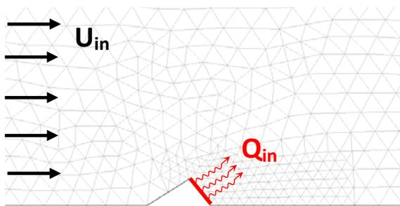
**Figure 6.** Geometry considered in the two-dimensional numerical simulation of the interaction between a lee-surface heat source and a lee-rotor. Significant boundary conditions are indicated:  $Q_{in}$  is the lee-surface input heat flux and  $U_{in}$  is the (constant) input air flow. The triangular mesh used to numerically solve the coupled fluid-heat conduction equations is also shown.
