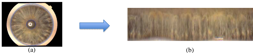
Figure 2. Iris Image Processing (a) Iris localization image and (b) Rectangular arrangement of the pattern.
