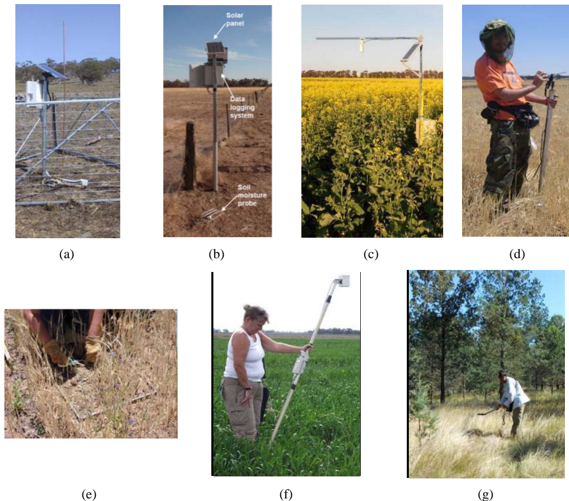
Figure 3. (a) Permanent, (b) semi-permanent, (c) supplementary stations; (d) HDAS for soil moisture sampling; (e)-(g) destructive, spectral and LAI vegetation sampling.
