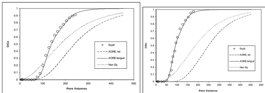
Fig. 3: The experimental data of fixed bed column tests and the breakthrough curves generated by various models at 20°C and 4°C.
