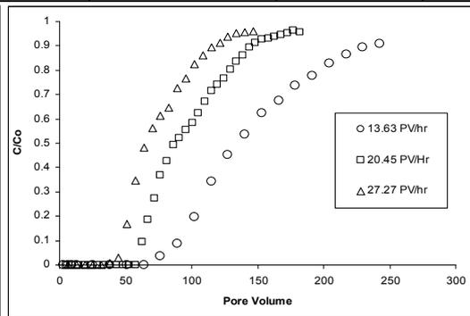
Fig. 1: The effect of flow rate on axial dispersion in packed column at 20<sup>o</sup> C. The lines represent the CXTFIT model fit.
