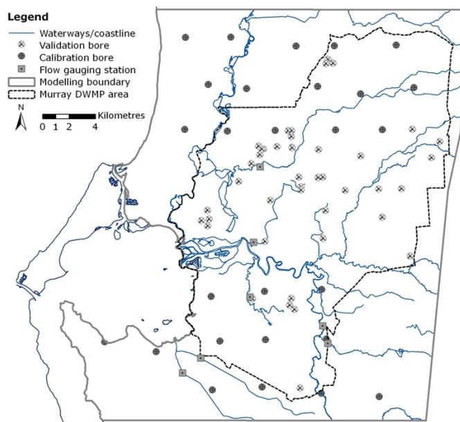
**Figure 4.** Calibration and validation groundwater bores and surface water flow gauging stations used in the Murray regional MIKE SHE model.
