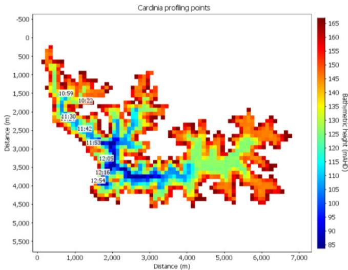
**Figure 2. Example of profiling points plotted on a bathymetric map of Cardinia Reservoir. The figure was generated using GPS coordinates in MW ARMS. Numbers of the format HH:MM indicate the time the profile was taken.**
