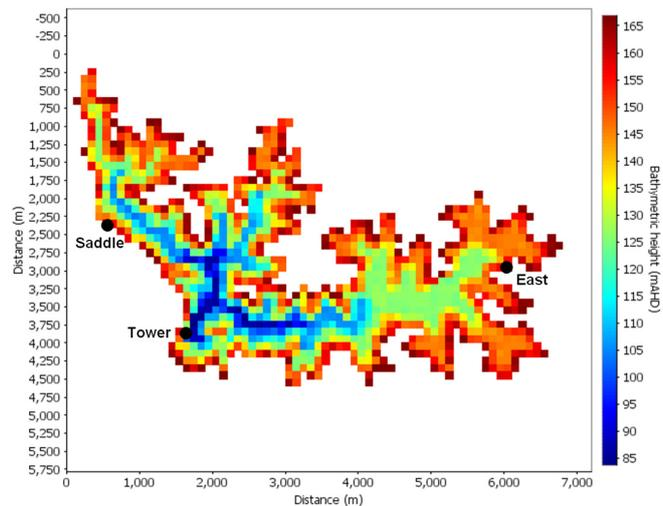
Figure 7. Cardinia Reservoir ELCOM bathymetry showing the three possible locations for desalination inflow: ‘Saddle’, ‘Tower’ and ‘East’. The colour bar is bathymetric height in m AHD, with dark blue indicating deep regions and dark red indicating shallow regions. After Yeates *et al.*, 2007.
