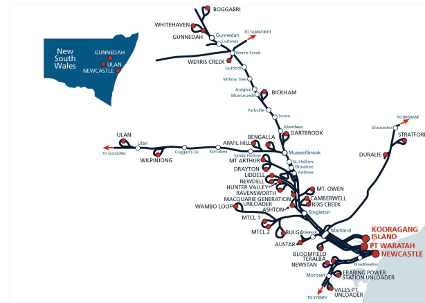
Figure 1: A schematic of the Hunter Valley coal chain (HVCC), showing rail track and the locations of mines and coal loading facilities
