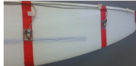
Figure 1.AUV's wing built with vibration sensors
