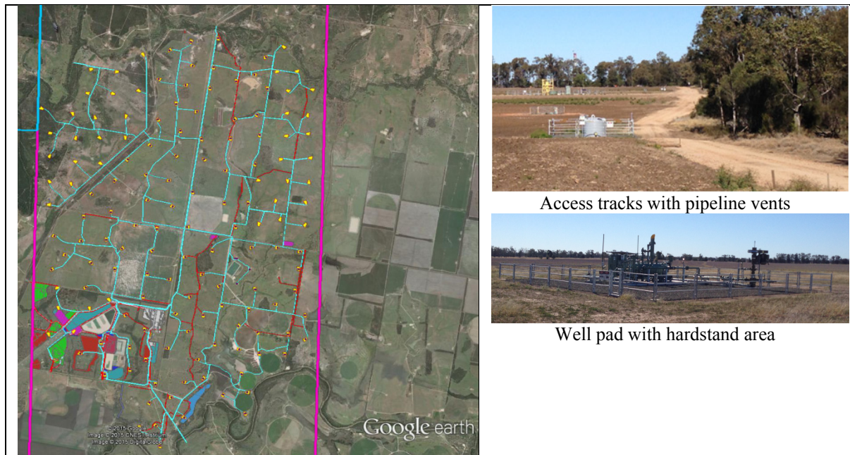
Figure 2. Left: CSG infrastructure network in the study area consisting of well pads, access tracks, gas treatment and water treatment facilities in the study area. E-W width of the development area ca. 8.3km, NS extent of the study area approx. 12km. Right: Example of an access track and a well pad in the field.
