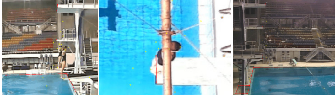
Figure 3. Cropped stills from each of the fixed video cameras with marked up landmarks. Red crosses indicate landmarks with known world coordinates ( x,y,z ). Yellow crosses indicate features that are simultaneously visible in multiple views but don't have known world coordinates. Red lines are drawn between adjacent landmarks.
