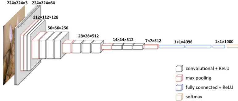
Figure 2. The architecture of VGG16 model (Shi et al. 2018).
