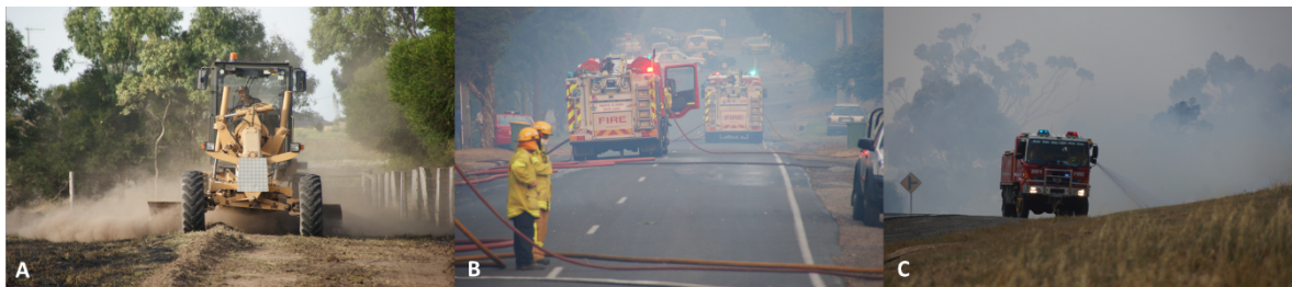
Figure 1. Example of three types of firefighting resources, including heavy plant in the form of a grader (pictured widening mineral earth control lines); a pumper appliance (deployed in the manner it typically would be for non-mobile asset protection); and a tanker appliance with a high capacity water tank being used for mobile ‘pump and roll’ edge attack
