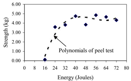
Figure 6: Relationship between weld strength and weld energy
