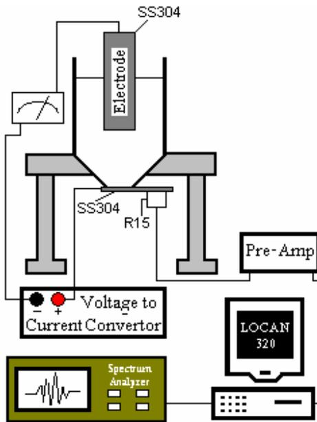
Figure 4: Diagram of AE system for corrosion monitoring
