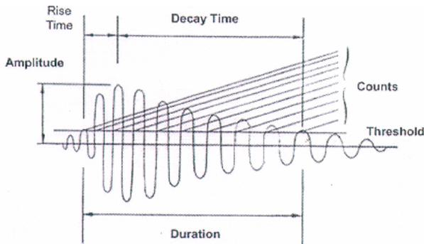
Figure 1: typical of AE parameter.
