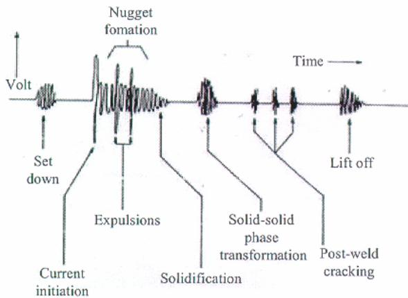
Figure 2: AE signal from spot welding process.
