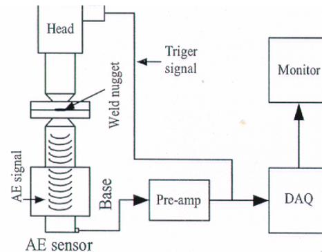
Figure 3: Diagram of AE system for spot welding monitoring
