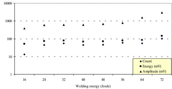
Figure 5: Relationship between AE parameters and different welding energy.
