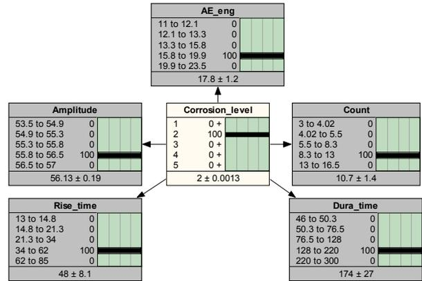
Figure 10: Belief network implemented to predict the probability of corrosion level.
