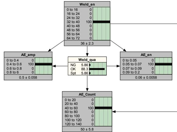
Figure 8: Belief network implemented to predict the probability of weld nugget quality.
