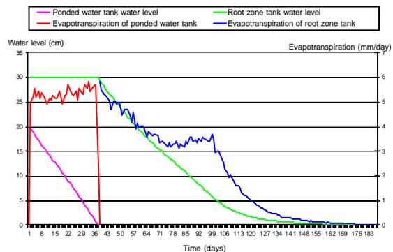
Figure 8: Verification of the evapotranspiration function at the simulated field level
