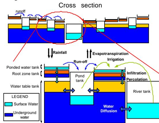
Figure 4: Structure and hydraulic functioning of the multi-agent model
