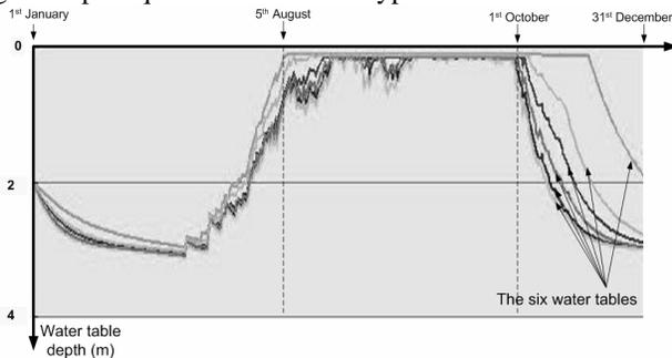
Figure 9: Calibration of the water levels in the six water-table tanks of the model
