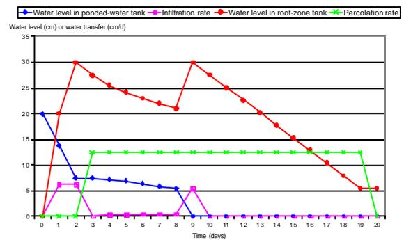
Figure 7: Verification of infiltration and percolation functions in a simulated field level
