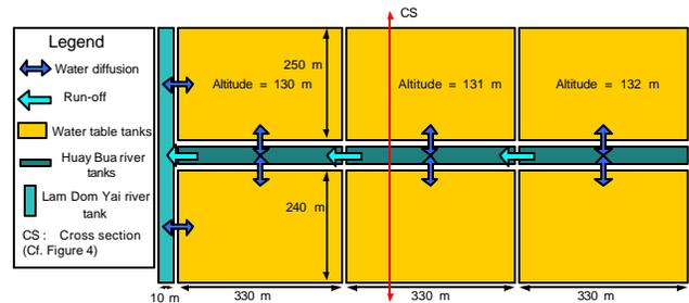
Figure 3: First layer of the model spatial entities representing the water table and rivers
